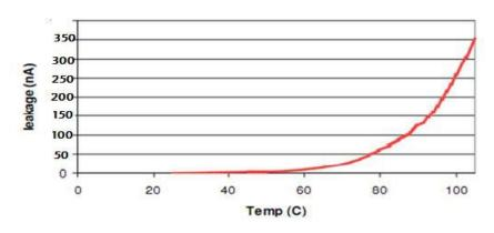
Fig4 Dark current temperature curve
