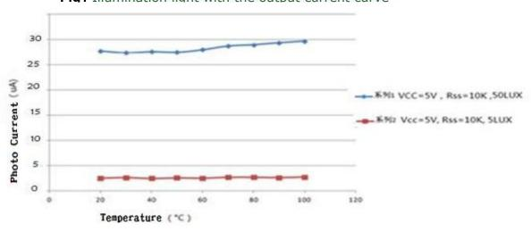
Fig2 Output light current changes curve with
