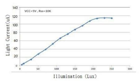
Fig1 Illumination light with the output current curve
