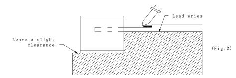
Regarding solution in the tinning oven for product-tinning, compound sub-solution made of tin & copper and sliver is proposed with the temperature of Celsius 260. The proportion of the alloyed solution is tin 95.5: copper 3.5: silver 0.5 by percentage. The time of tinning is constantly 3 seconds.
