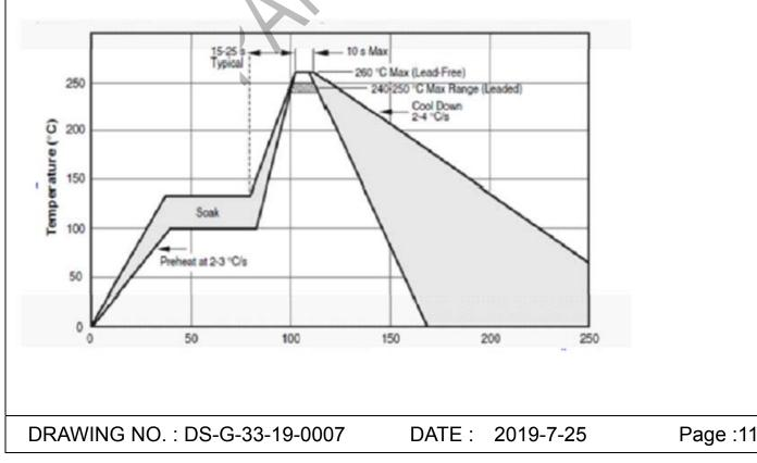
7) Recommended Wave Soldering Profile
