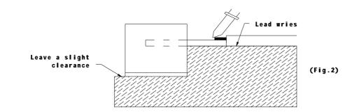
Regarding tinning the leads, compound made of tin ,copper and sliver is proposed with the temperature of  $260^{\circ}$ C. The proportion of the alloyed solution is 95.5% tin, 3.5 % copper, 0.5% silver. The time of tinning is 3 seconds.
