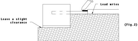
Regarding solution in the tinning oven for product-tinning, compound sub-solution made of tin & copper and sliver is proposed with the temperature of Celsius 260. The proportion of the alloyed solution is tin 95.5: copper 3.5: silver 0.5 by percentage. The time of tinning is constantly 3 seconds.
