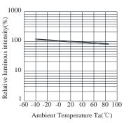
Fig.5 Luminous Intensity vs.Ambient Temperature
