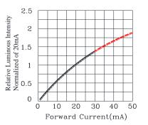
Fig.4 Relative Luminous Intensity vs.Forward Current
