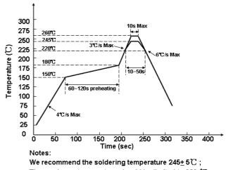
The maximum temperature should be limited to 260  $^{\circ}\mathrm{C}$ .
