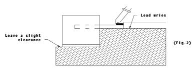
Regarding tinning the leads, compound made of tin ,copper and sliver is proposed with the temperature of  $260^{\circ}$ C. The proportion of the alloyed solution is 95.5% tin, 3.5 % copper, 0.5% silver. The time of tinning is 3 seconds.
